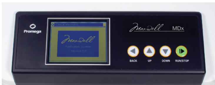
Figure 3. Touch Screen and Keypad. The touch screen and the keypad for use in navigating through the various screen displays for the Maxwell® 16 MDx Instrument. The same button selections are available on the keypad and the screen. Both sets of buttons can be used to navigate within and between screens. The Back and Run/Stop buttons allow navigation between screens. The Up and Down buttons are for navigation within a screen.
